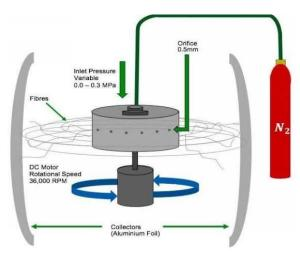
Figure 13: Pressurized Gyration
