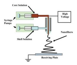
Figure 8: CO-Axial Electrospinning
