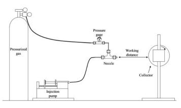
Figure 12: Solution and melt-blowing spinning
