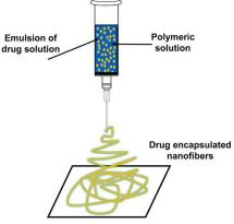
**Figure 7: Monoaxial Electrospinning**
