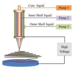
**Figure 9: Triaxial Electrospinning**
